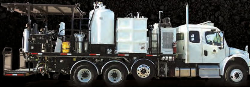
MRL MODEL 1-500-AA WATERBORNE PAINT STRIPING TRUCK
