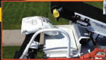
MRL MODEL 4-16000 THERMOPLASTIC STRIPER WITH CONVEYOR BAG LOADING
